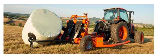
The Kubota Turntable wrappers can be fitted with a bale turner as an option.
