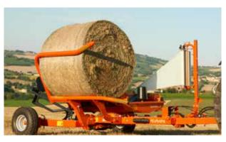
Hydraulically operated loading arm, with a low loading height, provides fast transfer of bale from arm to turntable.
