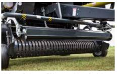
Kubota BV5160-BV5200 with 86" pick-up and roller wind guard.
