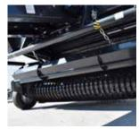
Clean raking 86" wide pickup with twin cam tracks, 5 tine bars and roller crop press.
