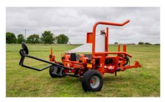
The loading arm is powered fully down to lift the wheel off the ground for easy movement from work to transport.
