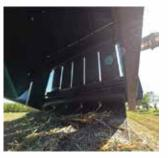
All balers come standard with Silage Scrapers meant for scraping build up of a wet or stringy crop around the rollers. This feature allows for use in dry or wet hay.
