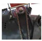
Main bale chamber drive is heavy duty 1 1/4" pitch chain.
