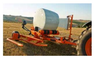
Turntable with two driven rollers designed for a high bale stability and smooth even rotation.
