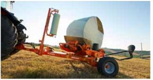
Low design of the machine ensures fast and gentle unloading of the bale.
