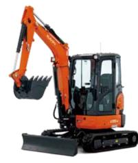
U35-4 🚇 🧀 Digging Depth: 9'8.9" (2,970 mm) Digging Radius at Ground Level: 16'11.3" (5.165 mm) 16'11.3" (5,165 mm)
