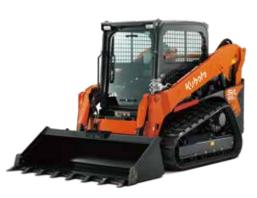
SVL65-2 Rated Operating Capacity @ 35% of Tipping Load: 2,100 lbs. (953 kg) Operating Weight: Open CAB 8,135 lbs. (3,690 kg) Closed CAB 8,631 lbs. (3,915 kg)
