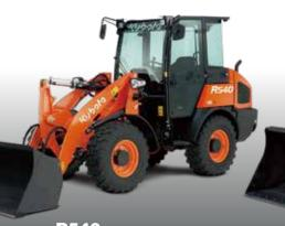
**R540** Operating Weight: CANOPY/CAB 9,888 lbs. (4,485 kg) / 10,285 lbs. (4,665 kg Bucket Capacity: 0.85 cu.yd. (0.65 m³)
