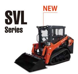
SVL50x Rated Operating Capacity @ 35% of Tipping Load: 1,176 lbs. (534 kg) Operating Weight: Open CAB 5,450 lbs. (2,472 kg) Closed CAB 5,620 lbs. (2,549 kg)
