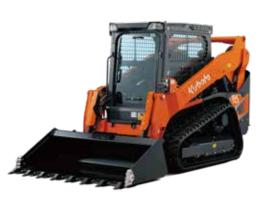
SVL75-3 Rated Operating Capacity @ 35% of Tipping Load: 2,490 lbs. (1,129 kg) Operating Weight: Open CAB 9,190 lbs. (4,169 kg) Closed CAB 9,420 lbs. (4,273 kg)
