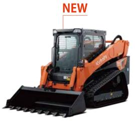
**SVL97-3** Rated Operating Capacity @ 35% of Tipping Load: 3,459 lbs. (1,569 kg)
