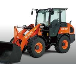
**R640** Operating Weight: CANOPY/CAB 11,177 lbs. (5,070 kg) / 11,563 lbs. (5,245 kg) Bucket Capacity: 0.94 cu.yd. (0.72 m³)
