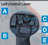
A. Horn B. –Not used– C. AUX1 D. AUX3 or Turn Signal E. Travel Speed
