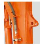
The factory-installed thumb bracket and relief valve significantly reduce the time needed to mount the optional hydraulic thumb.
