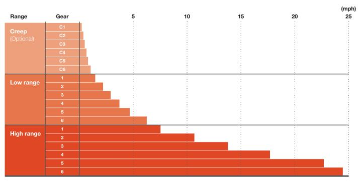
\*When H6 gear is selected, over drive function limits the maximum engine revolutions at 1960 rpm for better fuel economy
