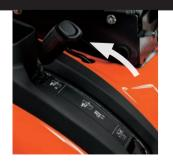
Pull the lever to lift the deck
