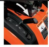
Release the lever to lower the deck
