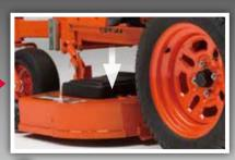
Push and release the pedal again to lower the deck
