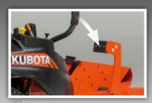
Push and release the pedal to raise the deck
