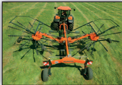
RA2076 - The hydraulically adjustable rotors can be set between 23'...
