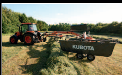
With 20" lifting height, swaths are easily crossed.
