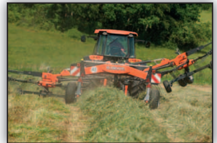
Single activation of rotors, has ability to rake the crops away from fence lines.
