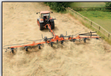
For border tending, the outer rotors are pivoted, to allow for an even inward spread of material.
