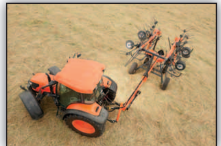
80° turning angle ensures excellent maneuverability.
