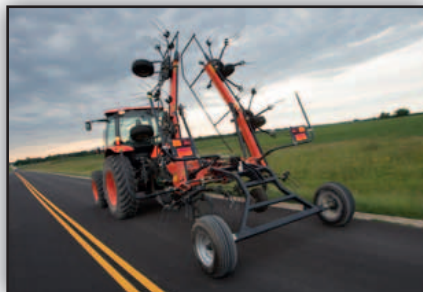
In transport position the weight of the carrier frame rests on the center part of the machine and the tractor drawbar.
