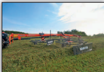
Center of gravity is close to the ground, allowing for excellent stability.
