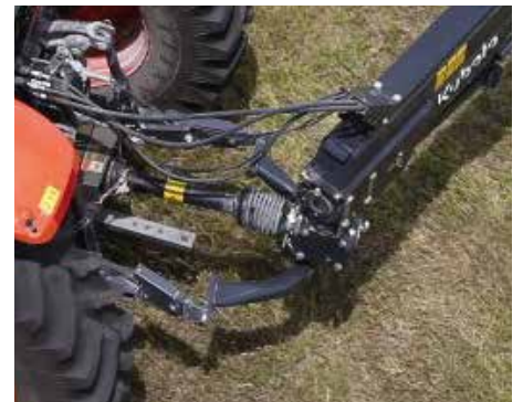
The swivel hitch headstock with reversible gearbox provides optimal maneuverability.
