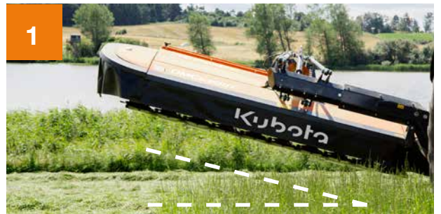
1 Minimum 1'8" ground clearance across the complete mowing unit during headland turns. Mowing unit is raised and carrying arm tilted to a 10° angle.
