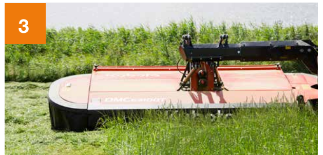
3 Mowing unit is lowered evenly onto the ground without one side touching the ground before the rest of the mower.
