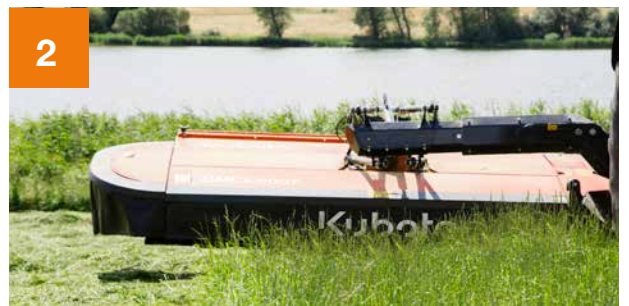
2 The carrying arm is tilted back to bring the mowing unit into an even position before lowering the mowing unit.
