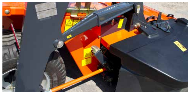
When an obstacle is encountered, the mowing section is forced backwards and the special suspension rod ensures that the mowing section is automatically lifted upwards and above the object.
