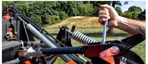
Stubble height adjustment is conveniently integrated directly into the suspension linkage. There is no need to tilt the A-frame of the tractor.
