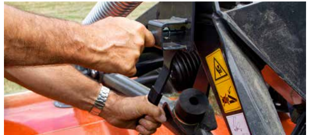
One-touch parking handle, to lock and prepare the machine for dismounting.
