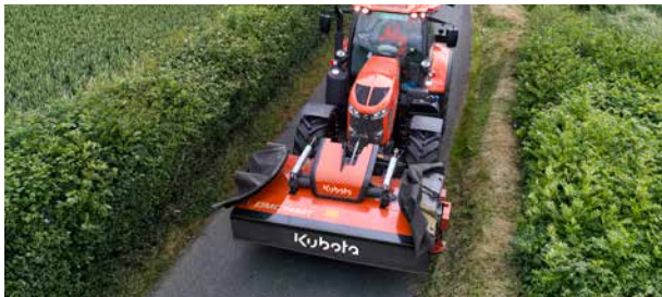
Hydraulic folding of FlexProtect guards (optional).
